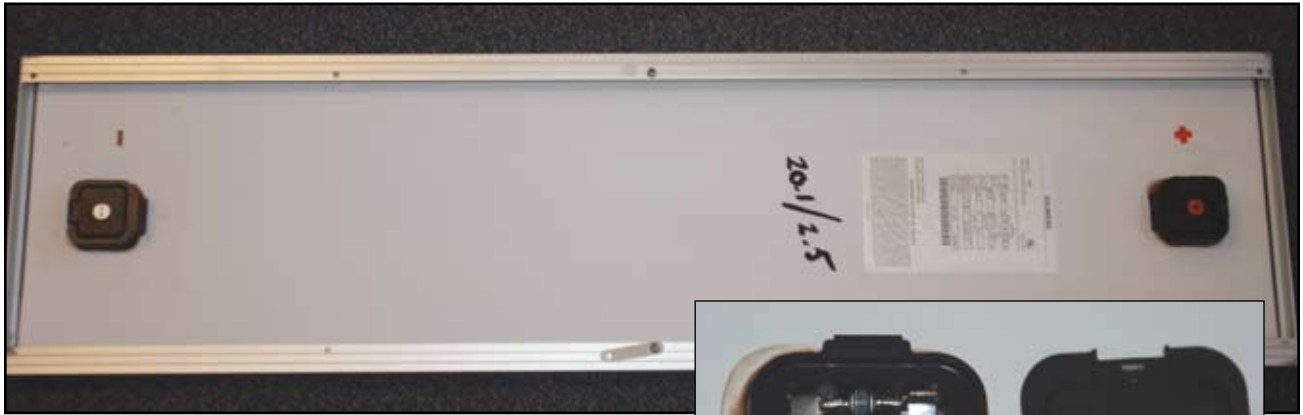
Photo 3. Older (1990s) PV module with two junction boxes
