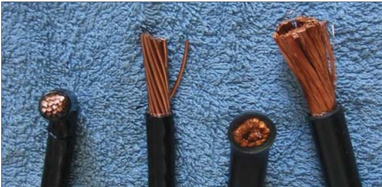
Photo 1. Standard Class B conductor (left) and fine stranded conductor (right)
