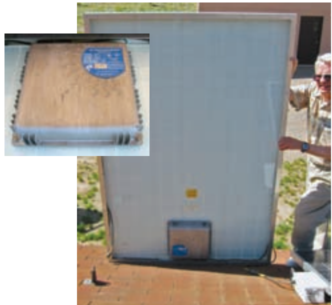
Grid-synchronous inverters integral to the module.
