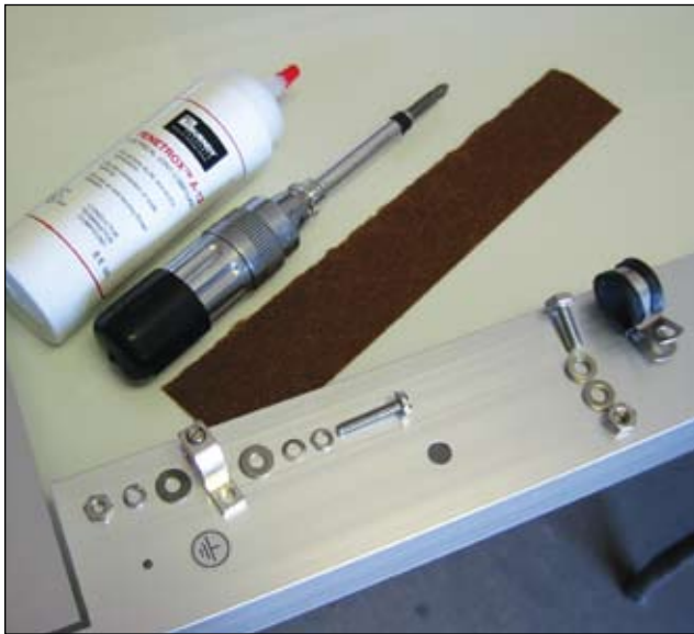
Photo 6. One module grounding method
