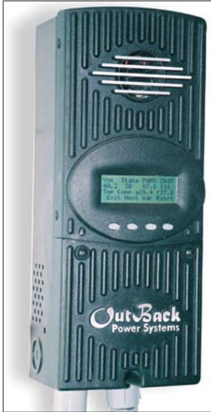
Photo 4. Battery charge controller
