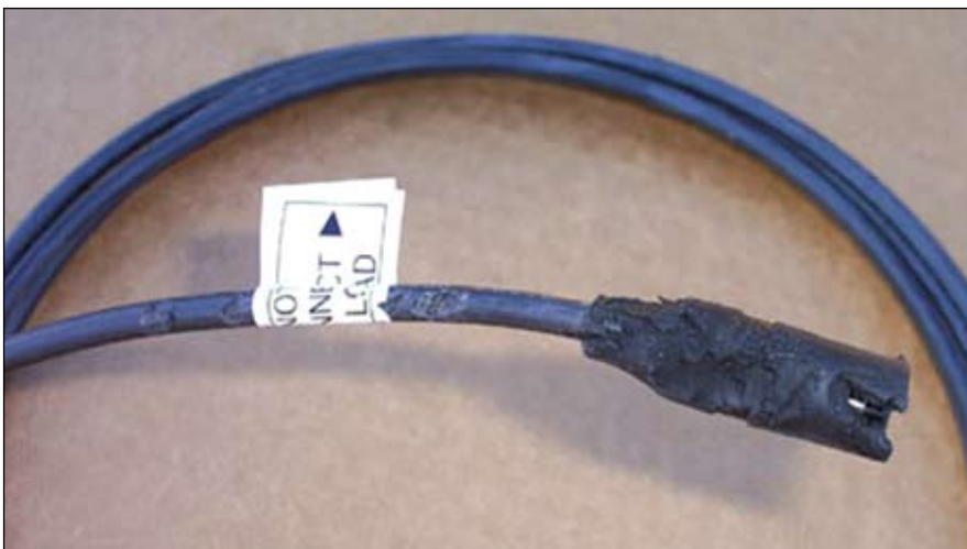
Photo 4. Rodent damaged cable and connector
