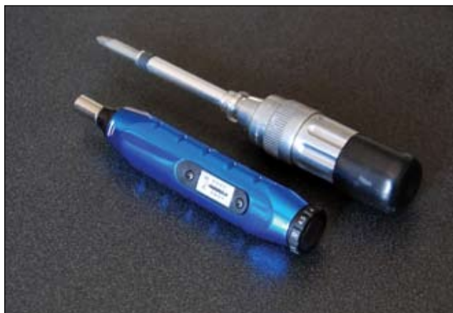
Photo 6. Torque screwdrivers are needed for electrical connections
