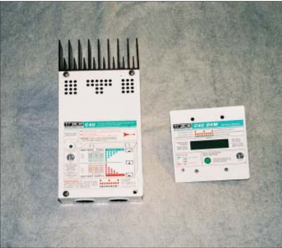
Photo 6. 40 A PV charge controller with remote display
